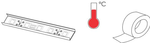
Use Aluminum profile or aluminum heat sink tape to avoid overheating, ensure proper heat dissipation and extend the life of the LED
