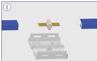
Connecting with interconnection connector
