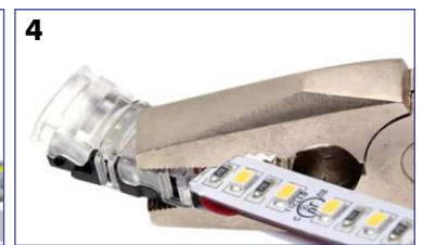
4 Complete the LED Strip connection using pliers. Make sure connection is locked at base of connector
