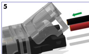
5 Insert 20 or 22 AWG wires into wire holder side of the connector
