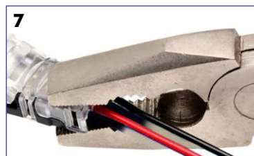
7 Complete the connection using Pliers. Make sure cap is locked at base of connector
