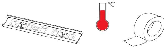
Use Aluminum profile or aluminum heat sink tape to avoid overheating ,
